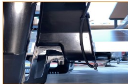
Examples of wire installation under FR510 Chassis.
