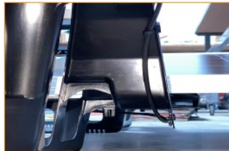
Examples of wire installation under FR510 Chassis.
