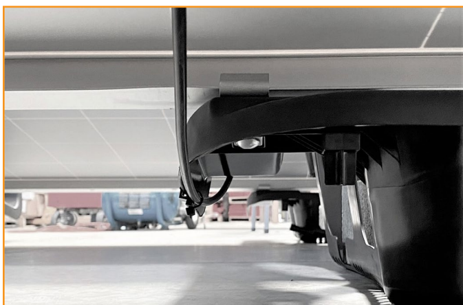
Examples of wire installation under BX Chassis.
