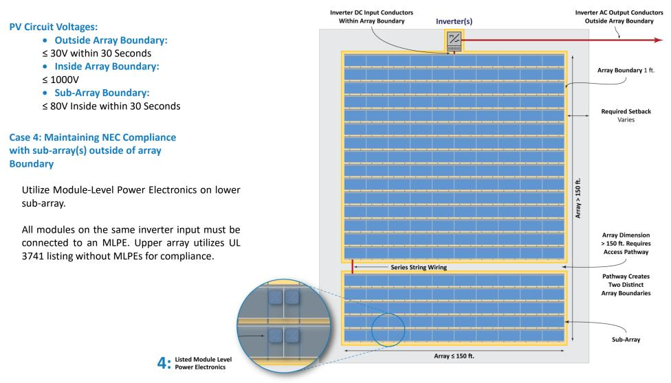
**ALERT:** When using MLPE devices, review installation instructions for both the MLPE device and Inverter to verify that both devices are compatible and comply with UL 1741 Rapid Shutdown requirements.
