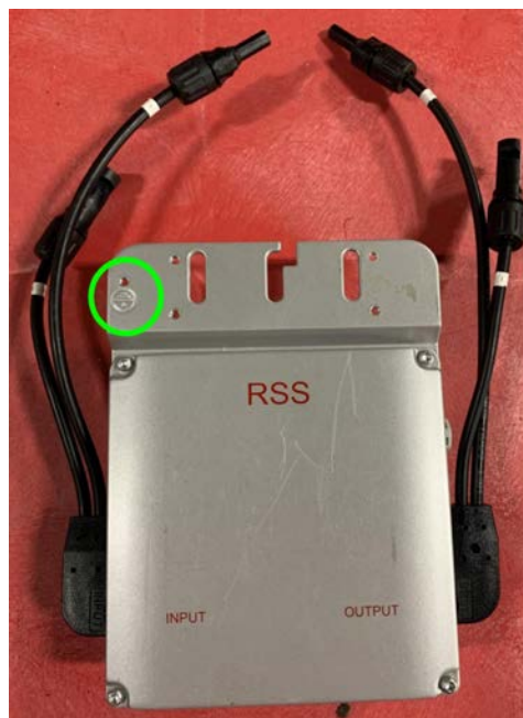
Figure 37. Smart RSS device showing M4 bolt
