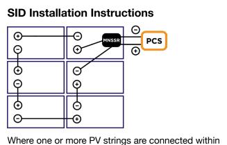
Where one or more PV strings are connected withir a single contiguous array as shown in the figure, the positive and negative ends of each string shall be connected to the MNSSR. The output conductors of each MNSSR get connected to the PCS. If there are multiple arrays, then each array each shall be equipped with an MNSSR as shown in the figure.
