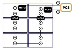
Where one or more PV strings are connected within a single contiguous array as shown in the figure, Tesla MCI-2s shall at a minimum be installed at both the positive and negative ends of each string between the last module and the homerun to the PCS. Two more MCI-2s are required anywhere within the string, but suggested to be placed between near ends of each string as shown in figure above.
