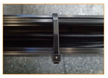
Install wires inside Aire Rail and install the Aire Wire Clip to retain wires inside channel, or use one of the approved Cable Ties to secure wires in channel. Where needed, cut off any remaining cable tie after installation. Modules must cover all wires after installation. There shall be no visibly exposed wires after installation of modules.
