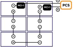
Where one or more PV strings are connected within a single contiguous array as shown in the figure, Tesla MCI-1s shall at a minimum be installed at both the positive and negative ends of each string between the last module and the homerun to the PCS. If there are multiple arrays each shall be equipped with MCI-1s as shown in the figure.
