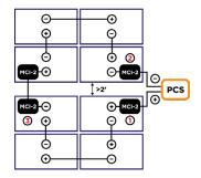
Where any string is connected across noncontiguous sub-arrays separated by more than 2' (see example figure), MCI-2s shall be installed as follows:
