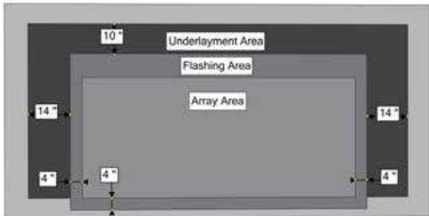
Location of Solstice Shingle™ Array Area
