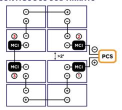
Where any string is connected across non-contiguous sub-arrays separated by more than 2' (see example figure), MCI-1s shall be installed as follows:
