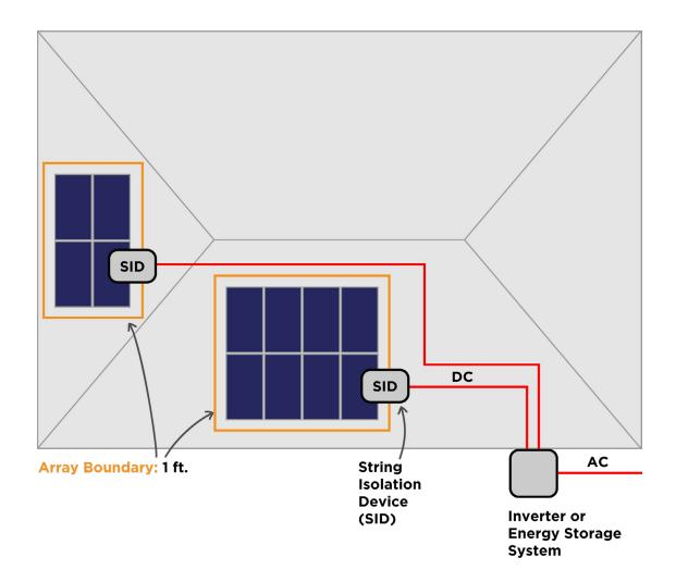
Case 3: Maintaining NEC Compliance with multiple arrays.
