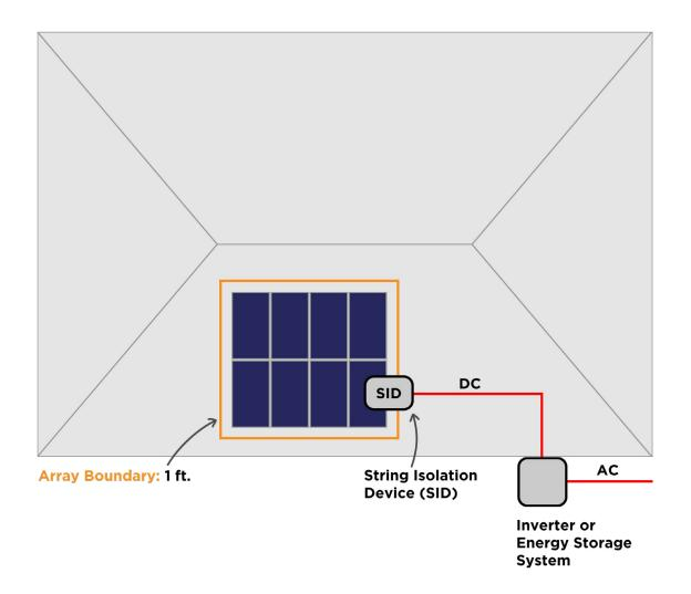
Case 1: Maintaining NEC compliance for single arrays.
