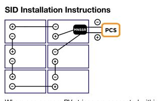
Where one or more PV strings are connected within a single contiguous array as shown in the figure, the positive and negative ends of each string shall be connected to the MNSSR. The output conductors of each MNSSR get connected to the PCS. If there are multiple arrays, then each array each shall be equipped with an MNSSR as shown in the figure.
