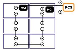
Where one or more PV strings are connected within a single contiguous array as shown in the figure, Tesla MCI-1s shall at a minimum be installed at both the positive and negative ends of each string between the last module and the homerun to the PCS. If there are multiple arrays each shall be equipped with MCI-1s as shown in the figure.
