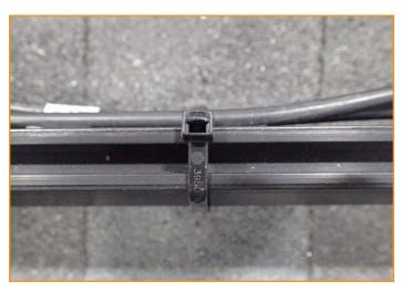
When running wires along the XR Rail, use the XR Wire Clip or the Cable Tie to secure wires to side of rail as shown above. Where needed, cut off any remaining cable tie after installation. Modules must cover all wires after installation. There shall be no visibly exposed wires after installation of modules. Do not overtighten or pinch the conductors.
