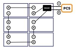
Where one or more PV strings are connected within a single contiguous array as shown in the figure, the positive and negative ends of each string shall be connected to the MNSSR. The leads of each MNSSR get connected to the PCS. If there are multiple arrays, then each array each shall be equipped with an MNSSR as shown in the figure.
